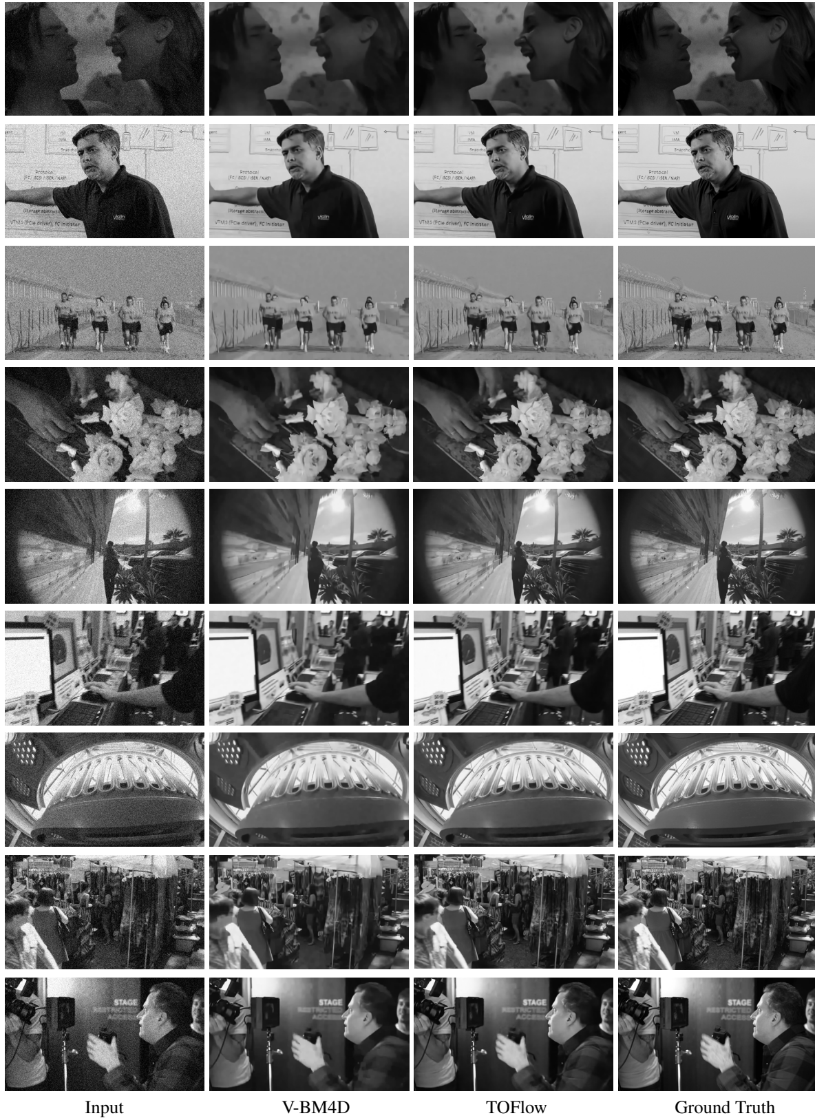
Fig. 16: Qualitative results on grayscale video denoising. Samples are randomly selected from the Vimeo denoising benchmark. The differences between different algorithms are clear only when zoomed in.
