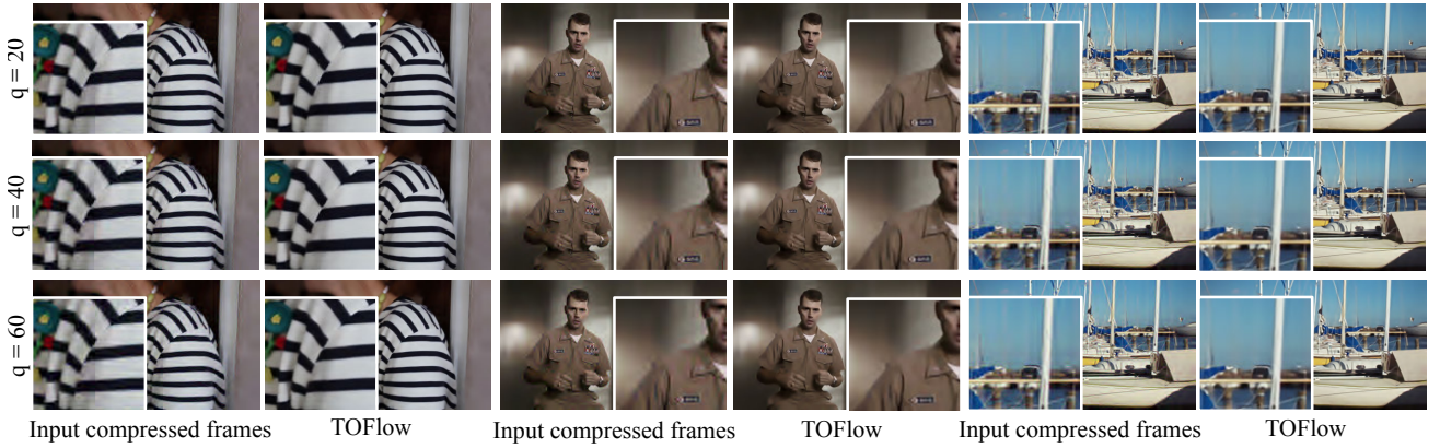
Fig. 10: Results on frames with different encoding qualities. The differences are clearer when zoomed-in.
